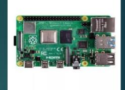
The "brain" running ROS 2. Options include compact boards like Raspberry Pi Raspberry Pi and Jetson Nano for embedded systems, or a laptop for more more powerful processing and development flexibility.
